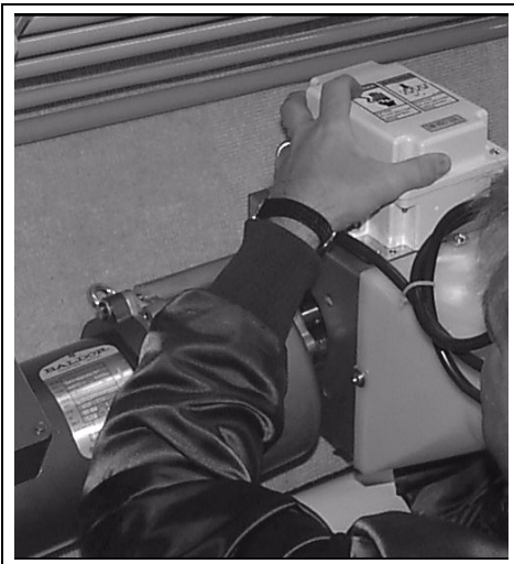
Figure 5R Assembly of the Control Unit to the Drive Unit
