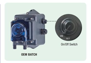
The custom OEM batch pump is factory programmed to run a specific length of time when manually activated by an integral switch or can be designed to activate with an input signal. The customer selects the pump run time from 0.1 seconds to 24 hours per activations.
